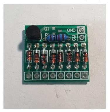
Before you start soldering, make sure that there are +5V on the 5V rail. So Either measure on the point where the 5V cable needs to be soldered to the UniPulse or on the cathode side (where the black ring is) of diode D45.
