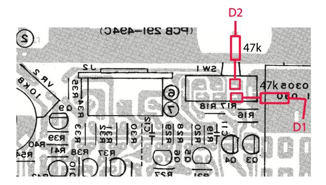
Attach two cables to D1 and D2 on the UniPulse and connect a 47k resistor to each end. The resistors than go to the two points shown in the picture above.
