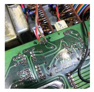
DC power is taken from the connector near the mains transformer, as shown in the picture. Ensure that RED goes to Ground, and BROWN goes to +8V. CHECK VOLTAGES FIRST! Trim the wiring neatly; there is very little free space inside the case with the baseplate fitted. Note that the baseplate has a foam cushion that bears against the backplane PCB to prevent shorts.
