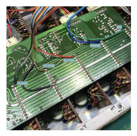
Next, attach the five drum trigger wires as shown. Note the labels on the drum channels. All the trigger connections are to pin 1 of each channel's edge connector. The curved black wire in the photo is a ground strap on this particular unit.
