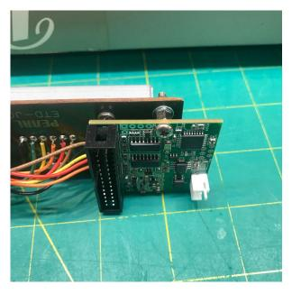
Then thread an M3 x 16 bolt through the uniPulse and tighten a 6mm hex spacer on the other side (see photos). Place a washer on either side of the connector PCB and secure it all with a nylock nut (again, see photos). Ensure the uniPulse is square with the connector PCB.
