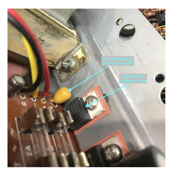
Once the regulator is changed, remount the regulators to the bracket, ensuring that you use proper insulated mounting kits. Note that the 7908 -8V negative regulator's fixing bolt MUST be insulated from the regulator; see the photo.
