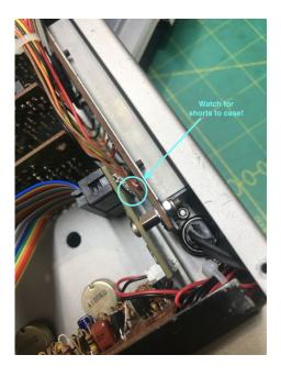
Now refit the connector PCB in the case, and attach the MIDI cable to the uniPulse, tucking the surplus wire well into the corner. You can now remount the remaining drum channel PCBs and the backplane PCBs, taking to care to align all the edge connectors. It's all pretty cosy.
