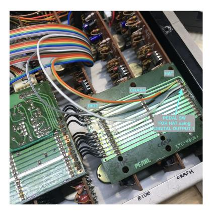
OUTPUT ONE (the next White wire) to control it. Although it is not shown in the photo, you will need to fit a BAT85 diode between the White wire and pin 3, with the cathode (ring) of the diode attached to the wire and its anode attached to pin 3. This ensures that the control line interfaces with the internal switching logic properly.
