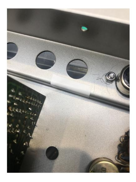
Place a small piece of PVC tape on the edge of the metalwork in front of the CYMBAL IN connector (see photo). There is a risk of the uniPulse's IDC header pins shorting against the case here, particularly if the hex spacer is 5mm or less.
