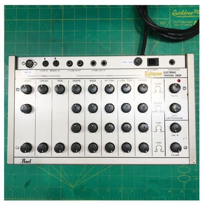
Mk3 or later; the Fightman only provides +/-8V DC rails, which are insufficient for powering earlier Mk1 or Mk2 uniPulse boards. Space is tight throughout the unit, so double-check all positions and measurements before drilling or cutting!
