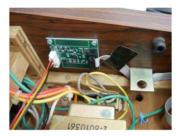
Mount the main board with the 2 2,9x6,5 screws as shown in the picture. It is advisable to mark the two holes with a marker and pre-drill a pilot hole. It is much easier to screw in the screws this way.
