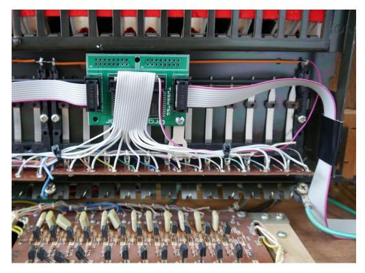
The red-striped wire is the common connection which gets soldered to the common bus bar in the upper right corner.
