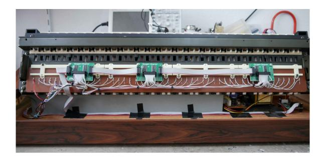
Install the interconnection cables and the switch cable assemblies.
