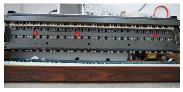
Next you need to cut away a bit of the rubber strip directly under the keyboard connector. This is where the common connections get routed to the connector.
