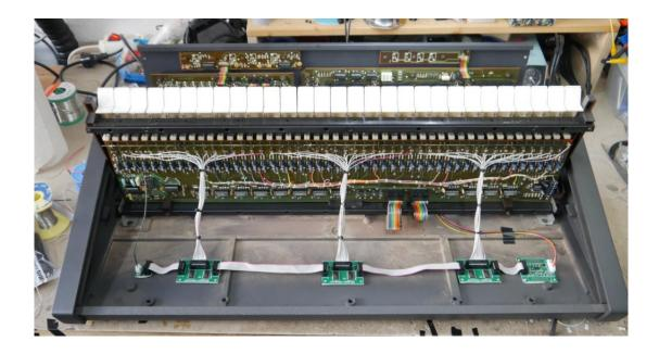
Plug in the interconnection cables between the boards.
