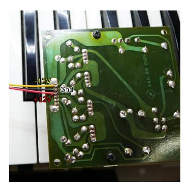
Solder the wires of the power cable assembly as shown in the picture. Take care not to create solder bridges.
