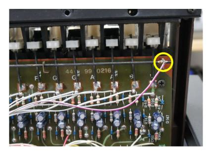
Wires 2 gets cut. Wires 3-18 get soldered to key contacts 49-34. Wires 19 and 20 get cut.
