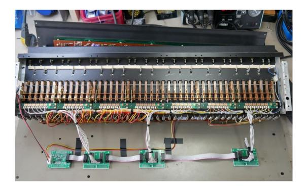
Plug in the interconnection cables and the switch board cables. Now solder the switch board wires to the key contacts:
