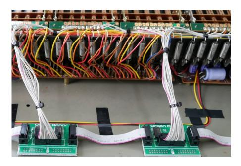
Then solder the wires to the power supply board.
