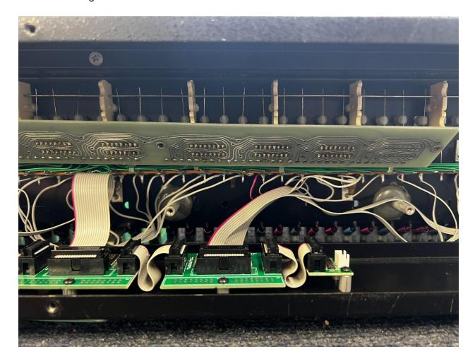
For the remaining switch boards, simply continue to solder to the base of the J wires.
