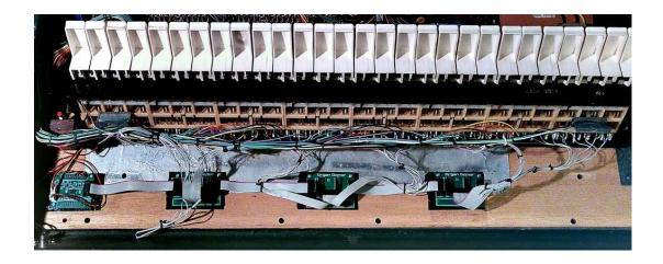
Plug in the interconnection cables and the switch board cables.
