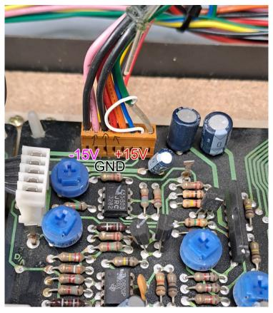
Remove the voiceboard, take care not to damage the plastic standoffs. Flip the voiceboard. Solder the power connections wires to the bottom side like shown. Plug the power wire assembly in the mainboard.
