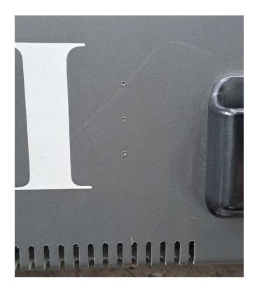
Drill the holes. 2X 3,2mm for the mounting holes, 15mm for the MIDI jack. For the 15mm hole you can either use a step drill or a screw holepunch. Install the MIDI jack and plug it in the main board.
