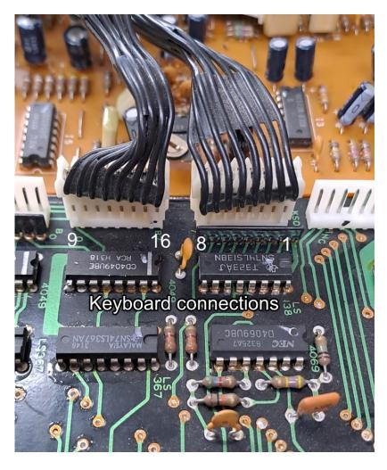
Remove the mainboard from the case and flip it. Plug in the 16pole ribbon cable to the matrix board. Solder the 16 wires of the ribbon cable to the bottom side as shown. Wire one is the one with the red stripe.
