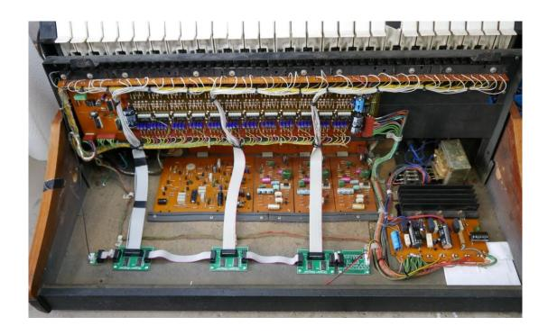
Mount the switch boards and the main board on the bottom plate of the synthesizer as shown in in the picture using the  $17\ 2,9x6,5mm$  screws. The rightmost and middle board have 16pin connectors, the large one on the left a 20pin connector. The leftmost board is a single switch pcb, especially for 49-key synths.
