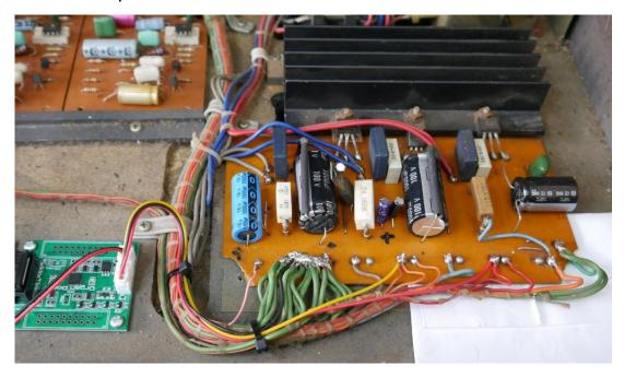
The black wire gets soldered to the green ground wires, the yellow wire gets soldered to the orange wires (-12V) and the red wire gets soldered to the red wires (+12V).
