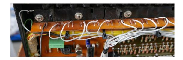
There are 2 diodes per key. The switch contacts get soldered to the anode of the right diode.
