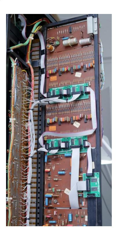
Install the interconnection cables and the switch cable assemblies. Cut the cables to length and strip the wires. Solder the wire to their respective points on the pcb.
