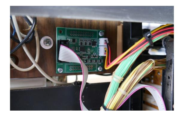
Extend the power wire assembly so the wires can reach the psu pcb. Plug in the power wire assembly and the MIDI wire assembly. Route the power wires to the power supply and solder the yellow wire to the -15V terminal, the black wire to the ground terminal, and the red wire to the output terminal of the voltage regulator you installed on the power supply board.
