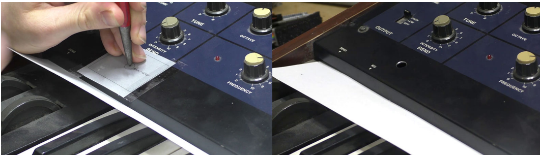
Figure 3: Drill guide placement, and hole drilling
