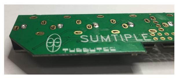
Use as little solder as possible or cut/pinch off the solder afterwards, so it looks like above. Check if the jacks are aligned, then you can solder the pins that are left, again, try to use as little solder as possible.
