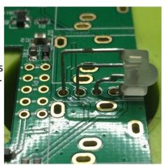
You can now place the 10-Pin-Header. Make sure it aligns with the board and solder two pins on every corner. Pinch off all pins so they only stick out a little.
