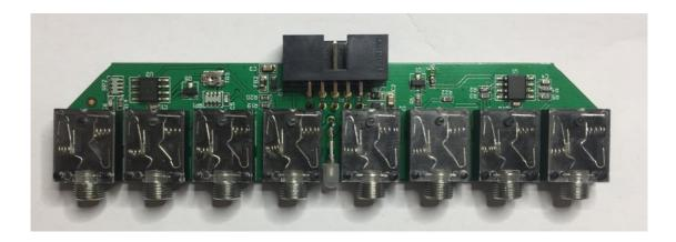
The Sumtiple is almost finished. The board should look like this now. You can take the front panel, attach it to the board and screw the nuts to the jacks.
