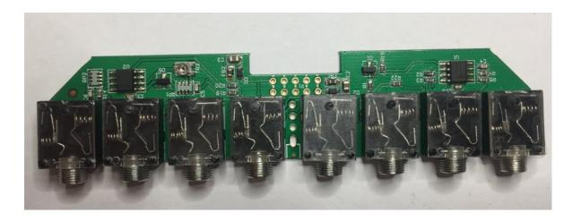
Now turn the board over. The easiest way, without all the sockets falling out, is to take a ruler and put it on top of the sockets, hold it with the PCB and turn it around. When you put it on the table, you can slide the sockets and PCB off the ruler.
