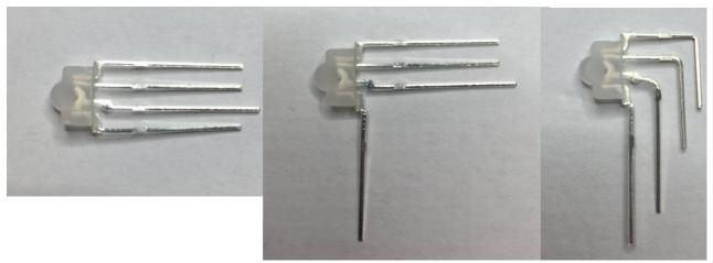
The flat side is looking towards you, note that one wire that is longer than the other three. The wire underneath it must be bend as near to the plastic part as possible.
