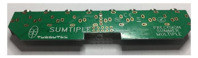
You can see that the pins are level with the PCB and not sticking out (This should be the case for every pin on the board [the LED and pin header pins]) Now start soldering one pin of each jack. That makes it easier to realign them before soldering the rest of the pins. We used the second pin from the left in the picture above.
