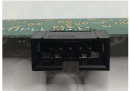
After pinching off the pins and soldering them, the pin header and the PCB should now look something like the right picture above.
