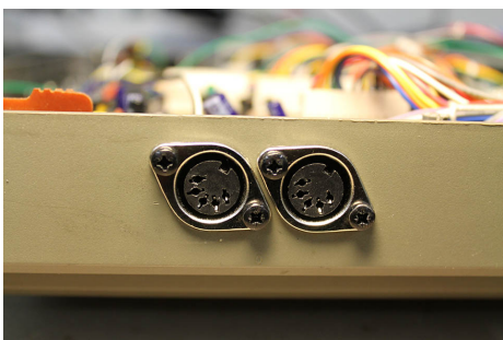
Figure 6: Holes drilled to final size and connectors installed
