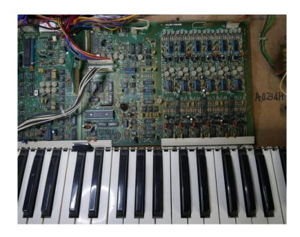
In order to install the processor board you have to remove the existing processor (IC6 D8049C 217) and replace it with the ModyPoly chip. You can use a small screw driver to carefully lift the processor out of its socket. When putting the ModyPoly chip into the socket, mind the orientation (cables are on the right side) and be careful not to bend any pins.
