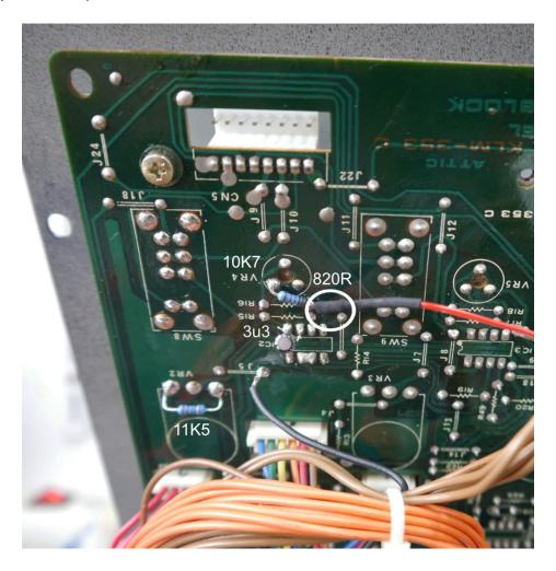
There are Mono/Poly's without screen printing on the board. In this case you need to take extra care where you solder the parts and wire to.
