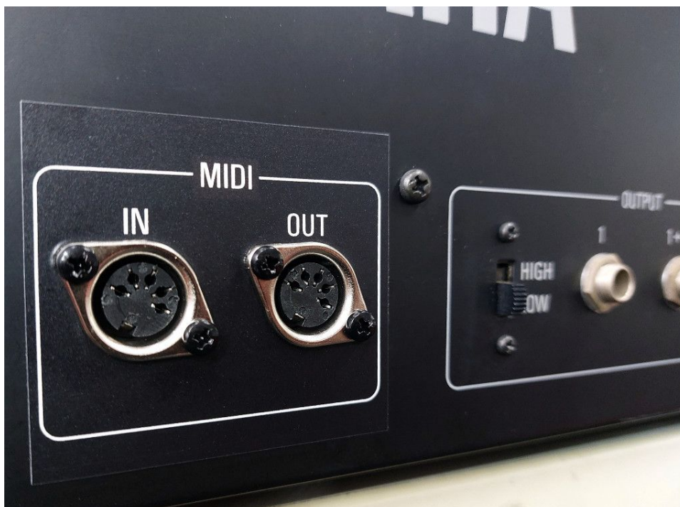
The installed MIDI sockets and overlay
