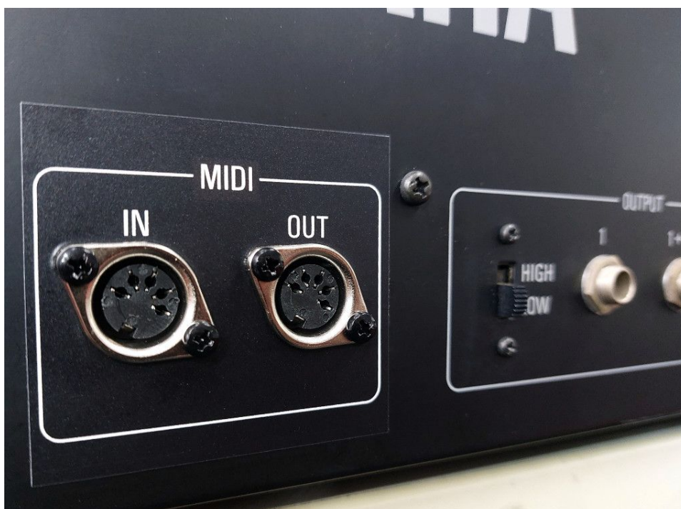
The installed MIDI sockets and overlay
