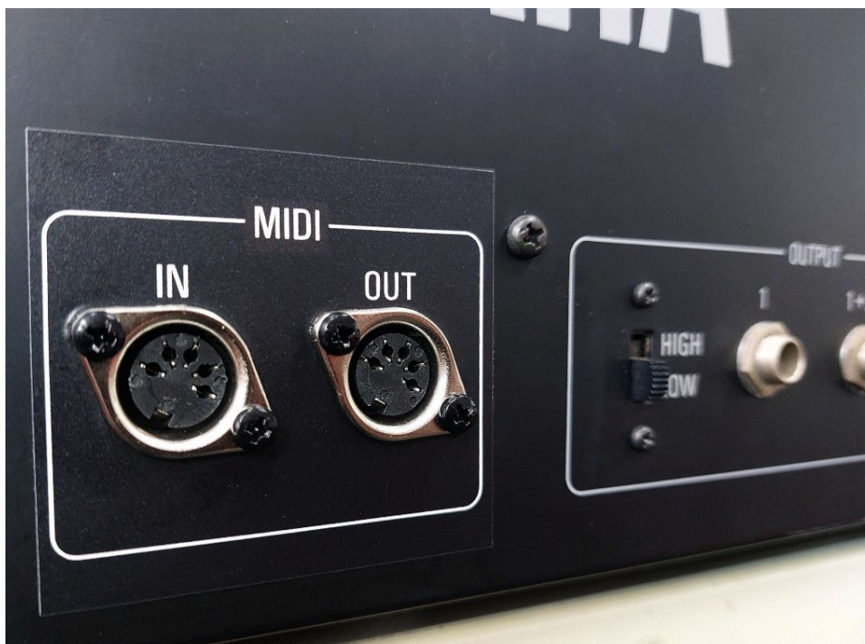
The installed MIDI sockets and overlay
