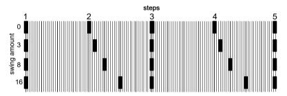
Swing amount can be set in the config menu by pressing FUNC + FWD and then selecting the amount from no swing ( AC ), to 16 ( LSTEP ).
